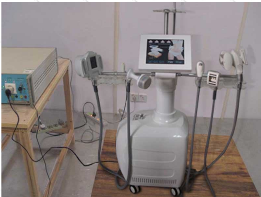
EFT IMMUNITY / SURGE IMMUNITY / VOLTAGE DIPS TEST SETUP
